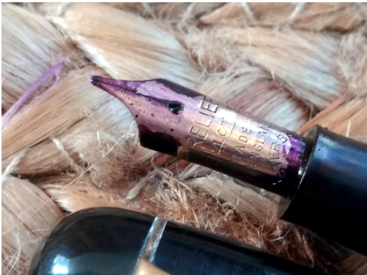
**Figures (4)** - The British Esterbrook Relief, manufactured by Conway-Stewart, 14K gold nib, lever fill.
