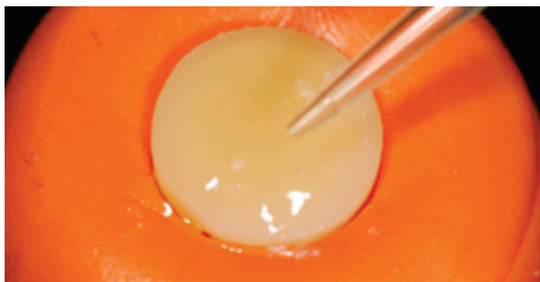
Figure 3 – Application of the hydrofluoric acid gel 10% (Dentsply) on the ceramic disc, which is wrapped by a silicone matrix so that the acid does not reach the opposite side of the disc.
